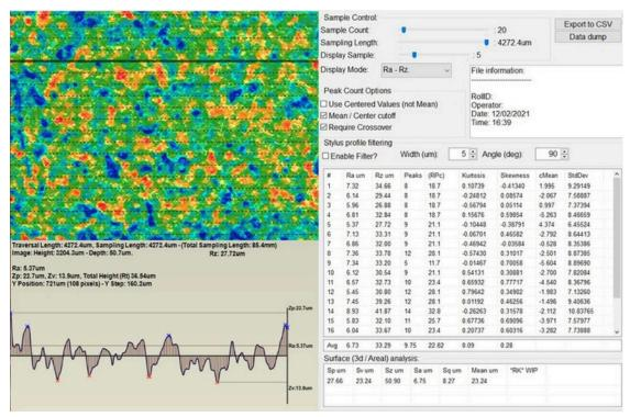
The RaRz Stylus profile lets users adjust the filter size (1-100µm) from the nominal 5µm, offering unrivalled sensitivity to surface roughness based on sample needs.
