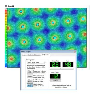
For opaque plates like letterpress and black elastomer, the system uses 3D data to capture what 2D imaging can't. It electronically slices the surface at a set offset, revealing dot shape, relief depth, and dimensions even when the top surface isn't clearly visible.
